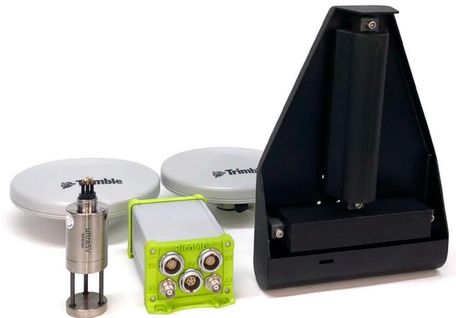
The PicoMB133 multibeam echosounder facilitates ultra-high resolution surveys on man-portable USVs and small survey vessels.
